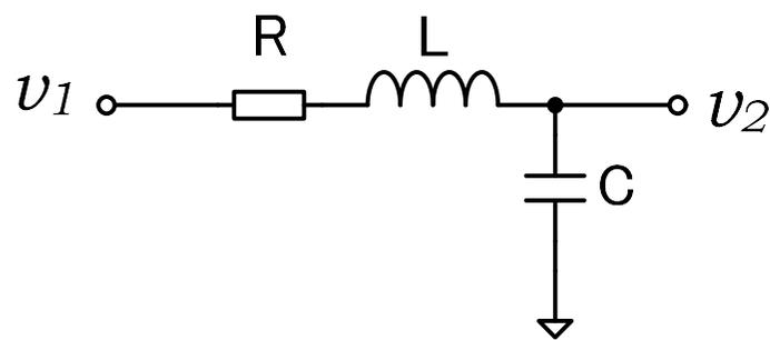
$$H(\omega) = \frac{\frac{1}{j\omega C}}{R + j\omega L + \frac{1}{j\omega C}} = \frac{1}{(1 - \omega^2 LC) + j\omega CR} = \frac{\frac{1}{LC}}{\left(\frac{1}{LC} - \omega^2\right) + j\omega \frac{R}{L}}$$
