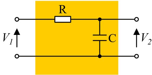
$$H(\omega) = \frac{V_2}{V_1} = \frac{\frac{1}{j\omega C}}{R + \frac{1}{j\omega C}} = \frac{1}{1 + j\omega CR} = \frac{1}{1 + j\omega/\omega_p} \quad (\omega_p = 1/CR)$$
